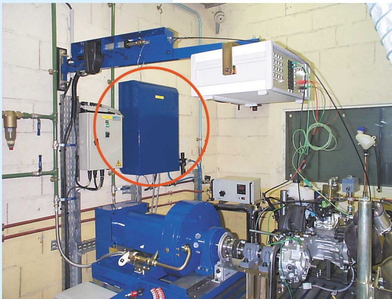
DMC 202 with its protection cover, installed in a test cell
